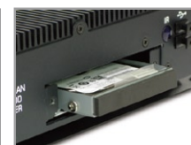
Removable / Anti-vibration HDD design
