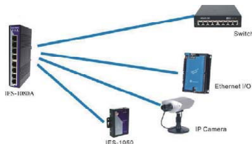
Connections of Ethernet devices
